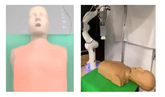
Robot-Assisted Autonomous Lung Ultrasound Scanning
