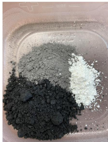
**Figure 1:** Combination of materials: paint sludge (gray), magnetite ore (black) and limestone (white).
