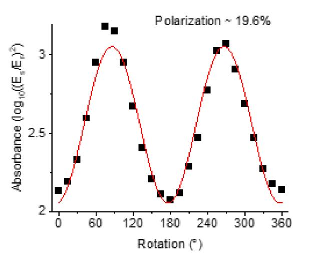
• Polarization is a measure of alignment that can be used in comparing yarns
