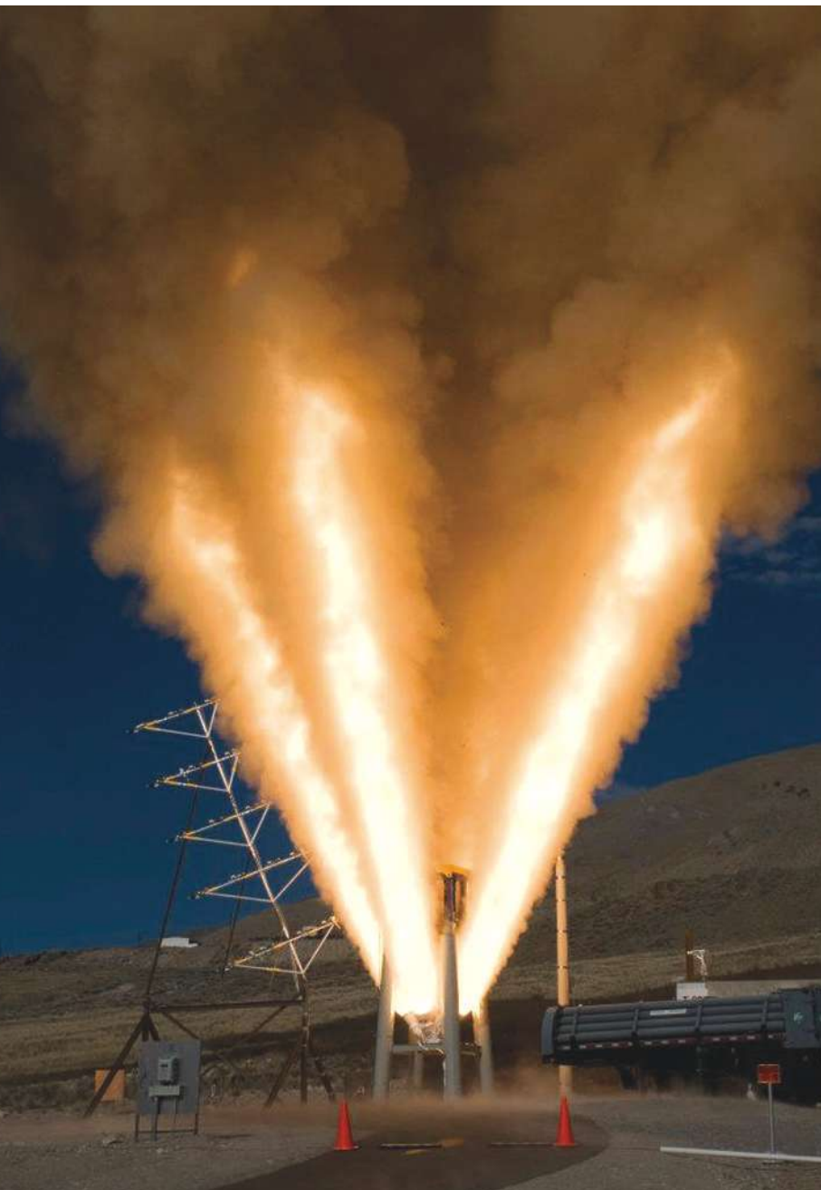
Successful ground test of the main abort motor for NASA's Orion Multi-Purpose Crew Vehicle.
