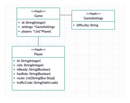
Figure 4.5: UML diagram of the Bus Bots redis data model
