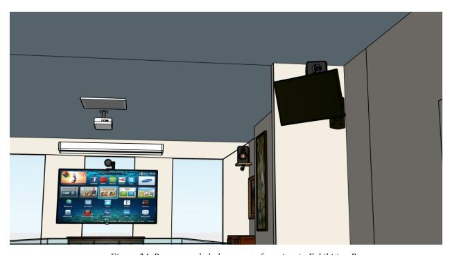
Figure 24. Recommended placement of monitor in Exhibition Room.
