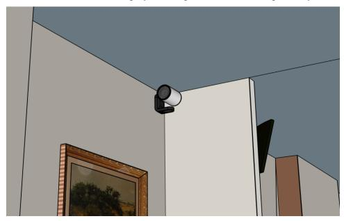
Figure 25. Recommended location of speaker-facing camera.
