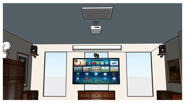
Figure 23. Recommended Video Room front configuration.
