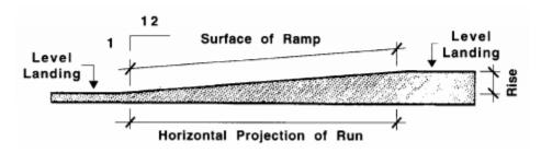
Figure 2.2 Example of a Curb Ramp Slope (Architectural Access Board: 521CMR, 2006)
