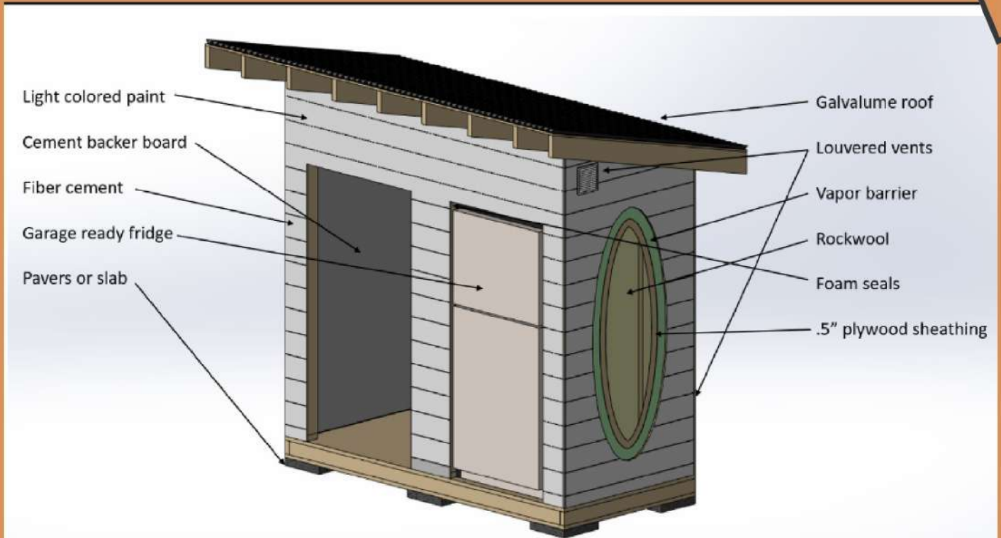
Figure 5.2 - Shows a 3D model representing the weatherization techniques of the budget design, the included weatherization solutions, and the wall composition for insulation as well as the cost breakdown.
