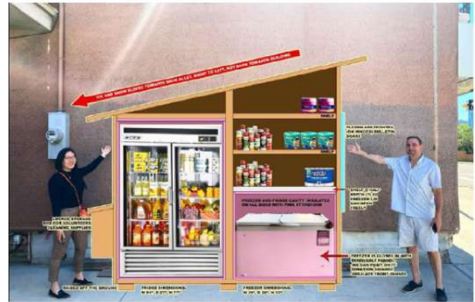
Figures 4.3, 4.4 – Basic guides for fridge building enclosures from programs in Regina and Calgary, Canada
