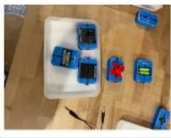
Simple Circuit Cubes: Small enclosed circuit components that children can make basic circuits with
