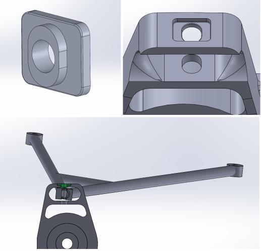
Figure 4: Camber block physical design solution
