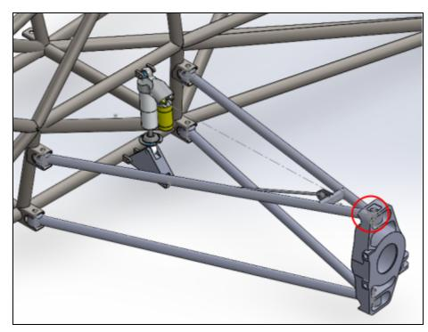
Figure 1: Camber block location in suspension system
