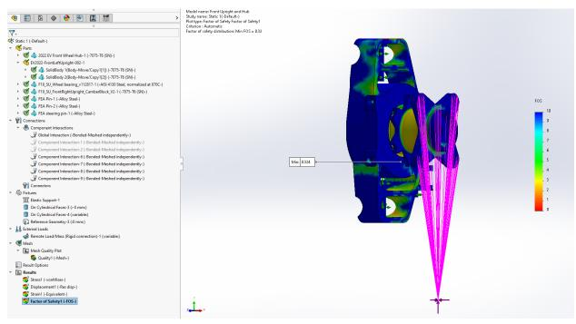
Figure 5: Upright assembly force element analysis
