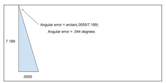
Figure 6: Error calculation from camber block tolerance
