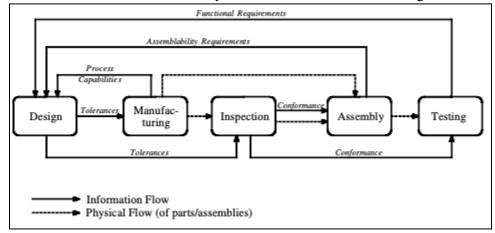
Figure 2: Traditional tolerancing method process flow
