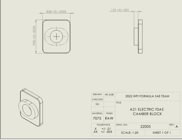
Figure 7: Technical drawing of camber block showing important tolerances
