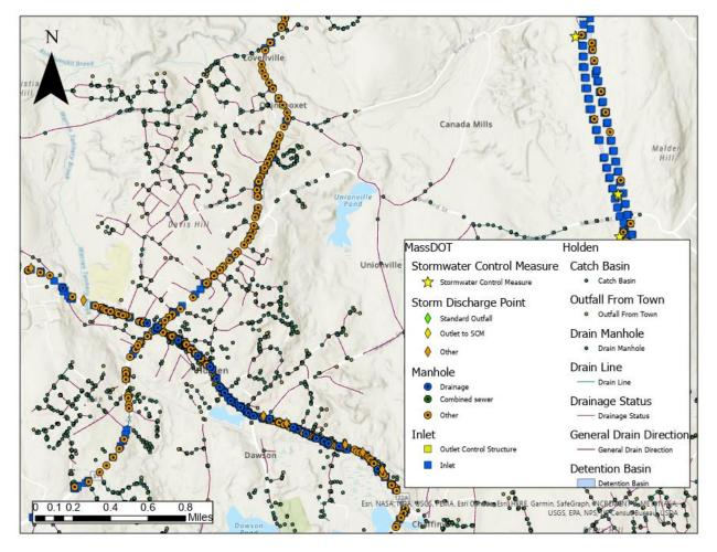
Figure 4.7 - Holden's and the MassDOT's MS4 Maps Overlaid
