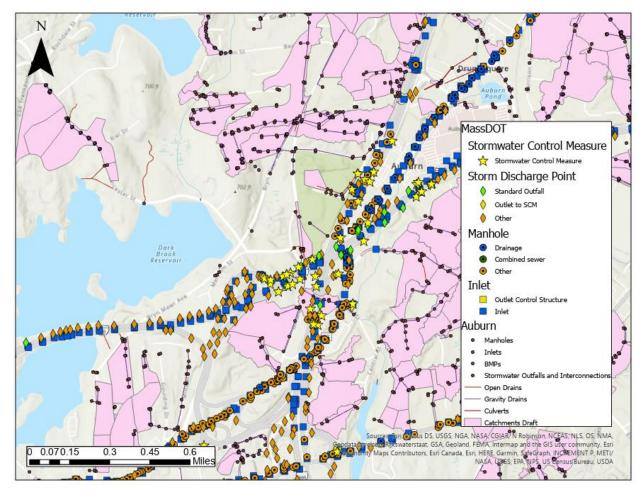
Figure 4.3 - Auburn's and the MassDOT's MS4 Maps OverlaidNote: The image above depicts the MassDOT's MS4 data overlaid on Town of Auburn's.
